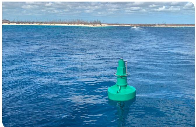
Every Sealite Marine Lantern, including the SL-70 (shown on the SL-B1750 buoy), flashes in unison with optional GPS sync.
